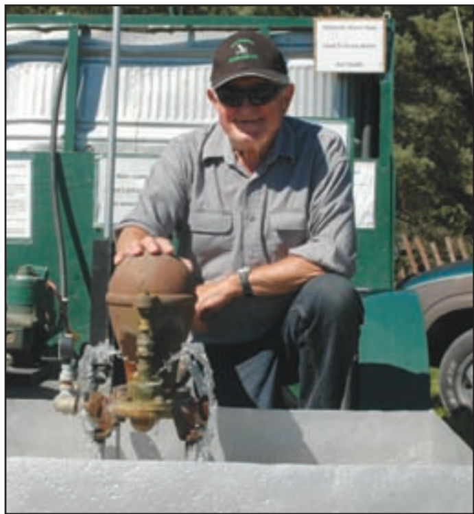
PHOTO BY BRIAN LOCKHART WORKING WATER PUMP – High County Antique Power Club member Earl Dodds, with his 1905 hydrolic ram water pump. The Club brought all sorts of old, but well maintained machines, for display at the 146th Annual Shelburne Fall Fair. Mr. Dodds pump is a working model that brought water to the second floor of the family farm house for 63 years.
