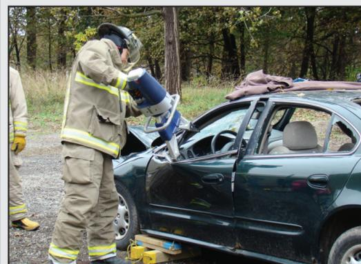
The Jaws of Life is a process involving several hydraulic tools specially designed to safely remove and injured or trapped individual from a car. From start to finish, brave Fire Fighters demonstrate the proper procedure to free an individual and save a life.
